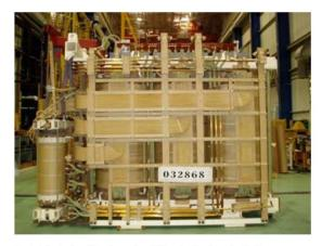
Prefabricated coil to clamp insulation is fitted on the bottom clamps prior to placing the coil assemblies concentrically on the core legs. The major insulation is usually of rigid form. It is prefabricated in a specially designated insulation area, isolated from other departments to provide carefully controlled clean and dry manufacturing and storage environment.
