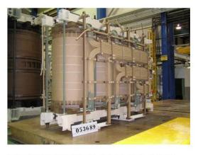
Increasing quality requirements demand a more and more careful treatment under vacuum. After the initially applied technologies such as the hot-air circulation process, the vaporphase drying process nowadays is the most efficient method to treat power transformers. At PTI Transformers LP we use a Hedrich system, 400 kW, cascade evaporator.
