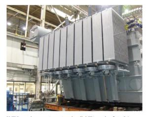
Utilities value assets, network reliability and safety. It is for this reason that PTI Transformer's design and manufacturing of utility grade transformers, (substation power transformers, auto-transformers and GSU transformers), are focused on having an unmatched low partial discharge (PD) of less than 25pC, when subjected to the induced voltage test per IEEE standard C57.12.00 and C57.12.90.
