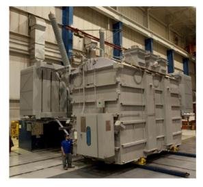
Transformer tanks are constructed of mild-steel and designed to withstand normal operating conditions, application full vacuum, lifting, jacking, and skidding.
