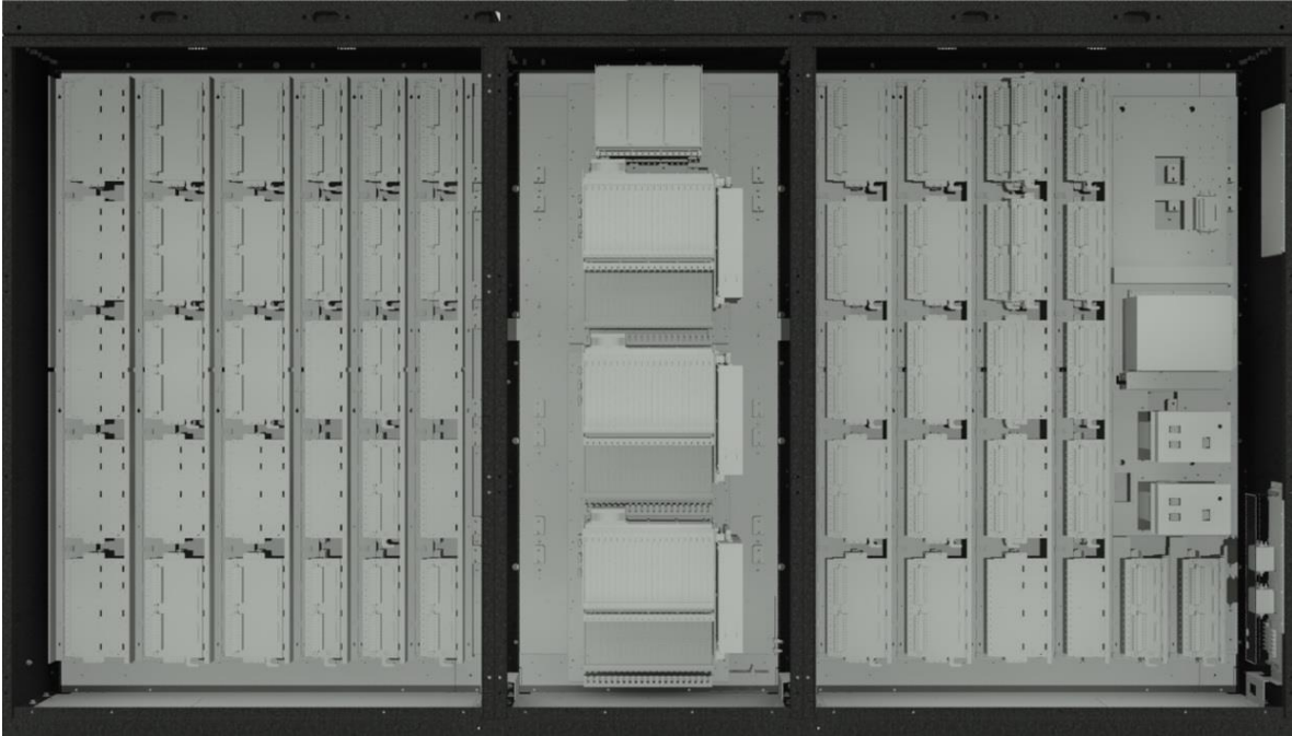
Today's TMR Mark VI Electronic Hardware Structure (Typical)
