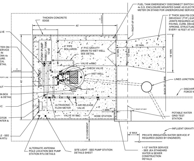
FOR PEAK FLOWS BETWEEN 0 TO 440 GPM
