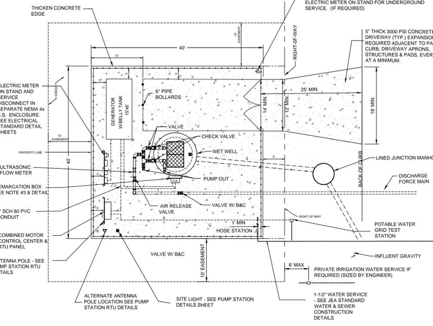
**FOR PEAK FLOWS BETWEEN 0 TO 440 GPM
