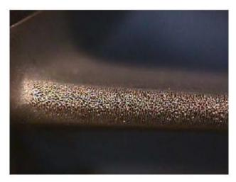
Figure 1: R0 leading edge erosion
