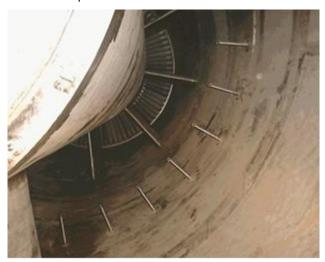
Figure 1. View of exhaust temperature probes, as seen when looking upstream into the exhaust.
