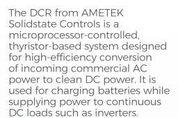
The rugged solid-state design utilizes SCR phase control to provide regulated, current-limited DC power. The DCR can operate with or without batteries and is intended for use in UPS systems. The DCR can also be used as a standalone device for battery-charging-only applications.
