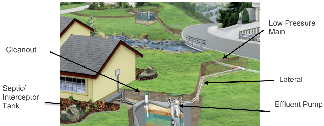
Figure 2-30: STEP Sewer Diagram (Orenco 2020)
