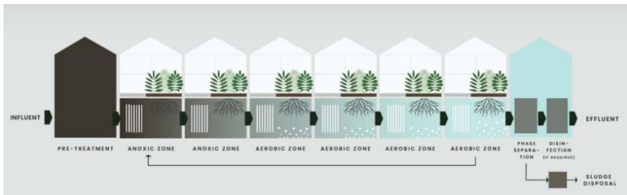
Figure 2-25: Proprietary Hybrid Constructed Wetlands System Process Flow Diagram (Organica)
