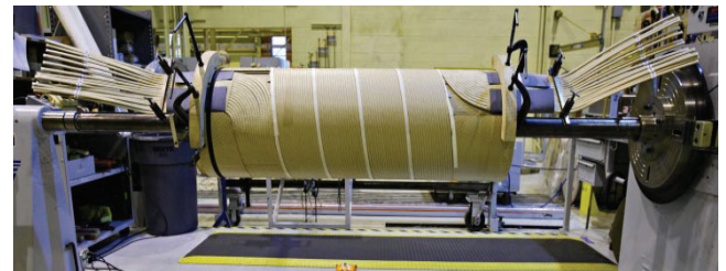
Fully Distributed Regulating Voltage Winding
