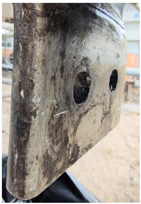
Contaminated conductor surface with evidence of heating.
