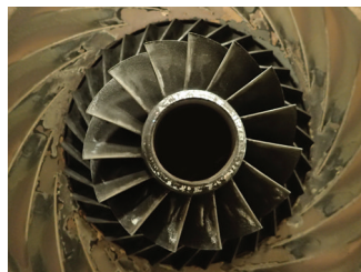
First stage impeller before and after overhaul.
