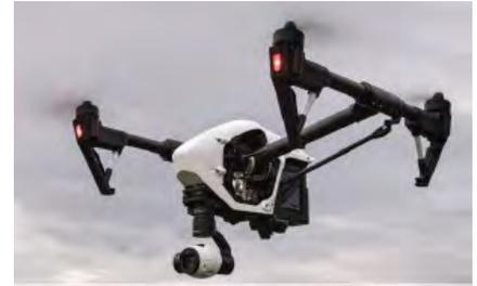
Pickett has been at the forefront of the UAS industry since 2015, and complies with all FAA regulations. We have since developed a system for capturing and processing imagery using Unmanned Aerial Vehicles (UAVs) outfitted with a high-resolution digital camera. This provides additional, affordable capabilities to augment our aerial mapping services.
