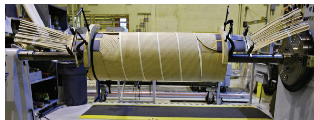
Fully Distributed Regulating Voltage Winding
