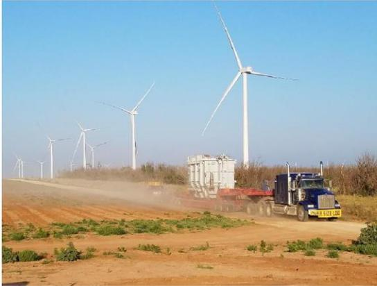
Medium and large power transformers by their size and weight are challenging to ship. The plant is ideally located to take advantage of both highway and rail links to major transportation arteries in North America. This allows PTI Transformers to ship transformers units to the four corners of the continent. PTI Transformers has significant experience in the transportation of large power transformers which reduces the risk of transportation damage for our customer.
