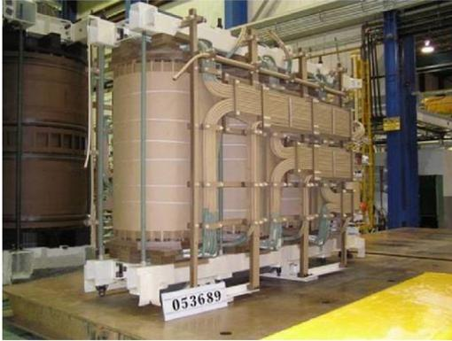
Increasing quality requirements demand a more and more careful treatment under vacuum. After the initially applied technologies such as the hot-air circulation process, the vapor-phase drying process nowadays is the most efficient method to treat power transformers. At PTI Transformers LP we use a Hedrich system, 400 kW, cascade evaporator.
