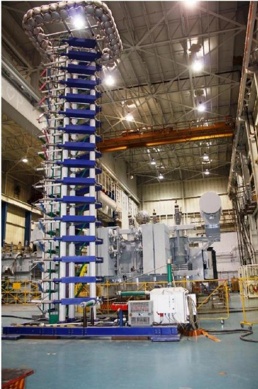
Prior to shipment, all transformers manufactured by PTI Transformers LP are tested in accordance with the latest applicable IEEE/ANSI and CSA standards and customer specifications.
