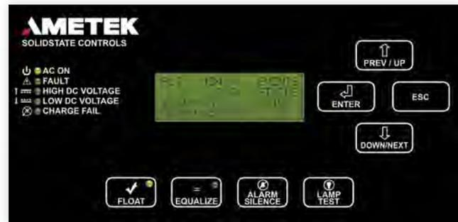
With the DCR's Digital Display, you have all the vital system information right at your fingertips. The user-friendly display menu provides the link between operator, all monitoring controls and alarms. Set points for control and alarm parameters are customer configurable.
