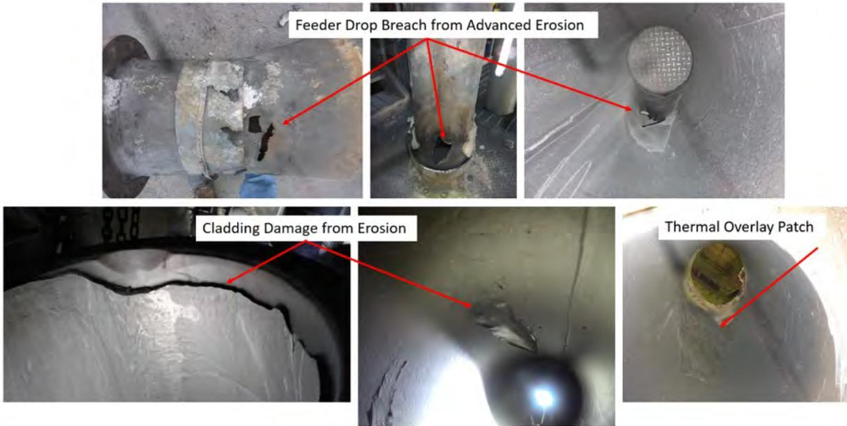
Although routine maintenance and repairs have been made to the drag conveyors over the equipment life, the rate of corrosion, erosion and fuel-based damage have surpassed the ability to repair as seen in Figure 7.
