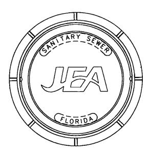
DESCRIPTION: Manhole Frame and Cover (with rubber "T" Gaskets). See Section 427 of the current JEA Standards for specifications and requirements.
