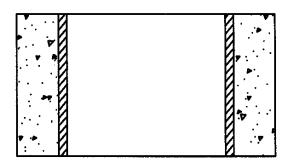
DESCRIPTION: Concrete Liner. See Section 446 of the current JEA Standards for specifications and requirements.
