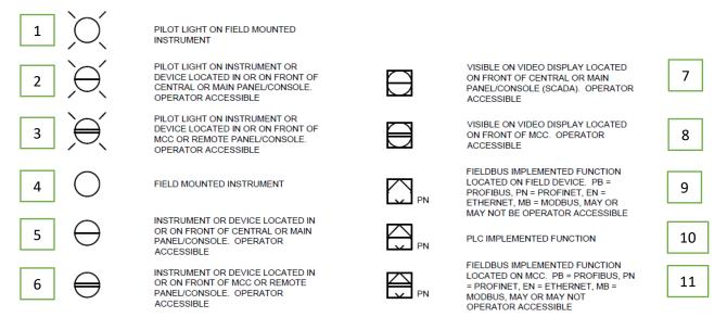
The GENERAL INSTRUMENT OR FUNCTION SYMBOLS chart is provided as guide to indicate and locate instruments in the drawing set.
