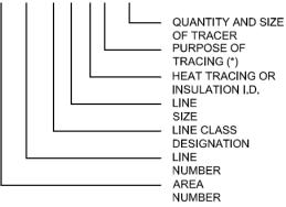
HEAT TRACING AND INSULATION I.D.
