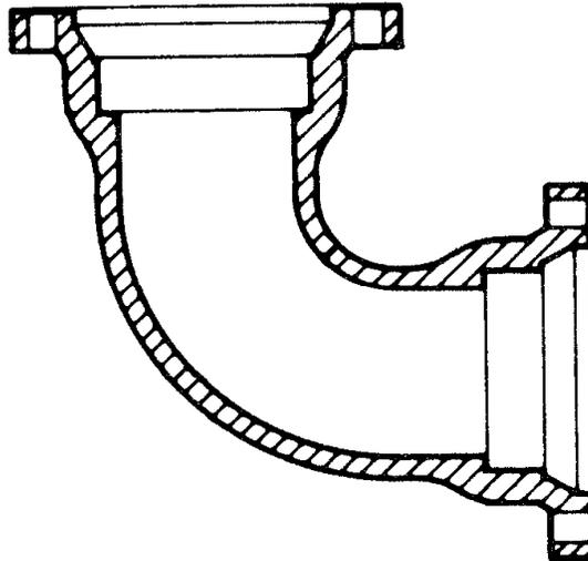
**Note:** Mechanical Joint, 90-degree bend, **shown** as example only (for additional joints & fittings, see specifications).
