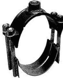
**Note:** Select desired saddle O.D. range which specifically matches outside diameter of pipe. Saddles for C-900 shall be sized to the exact O.D. size for proper fit. A double strap saddle will be required for all wet taps and are acceptable for installation on dry water supply mains (all sizes).
