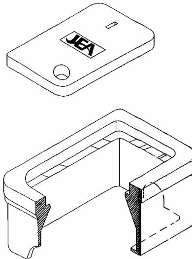
**DESCRIPTION:** Meter Box. See Chapter III. 2. - Section 351 of the current JEA Standards for specifications and requirements. See Chapter V. 2. - Section 702 for Reclaimed Water specifications and requirements.
