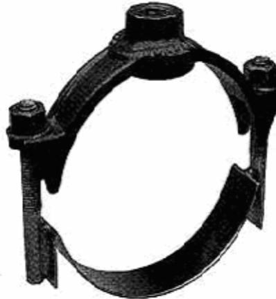
**Note:** Select desired saddle O.D. range which specifically matches outside diameter of pipe. Saddles for C-900 shall be sized to the exact O.D. size for proper fit. Single Strap Saddle is approved for new 1-inch water services only which are installed on dry water main, sized 4-inch through 10 inch.
