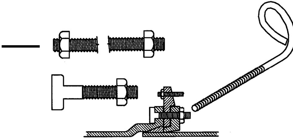
**DESCRIPTION:** Mechanical Joint Fasteners. See Chapter III. 1. - Section 350 of the current JEA Standards for specifications and requirements. See Chapter VI. 1. - Section 701 for Reclaimed Water specifications and requirements.
