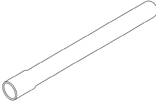
**DESCRIPTION:** PVC SCH 40 & SCH 80 Pipe. See Chapter III. 1. - Section 350 of the current JEA Standards for specifications and requirements. See Chapter VI. 1. - Section 701 for Reclaimed Water specifications and requirements.
