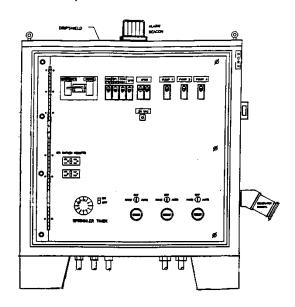
**<u>DESCRIPTION:</u>** Pump Station Electrical and Control Panel including (RTU). See Section 433 of the current JEA Standards for specifications and requirements.
