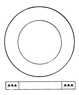
**DESCRIPTION:** Manhole (adjustment rings) Collars. See Section 427 of the current JEA Standards for specifications and requirements.
