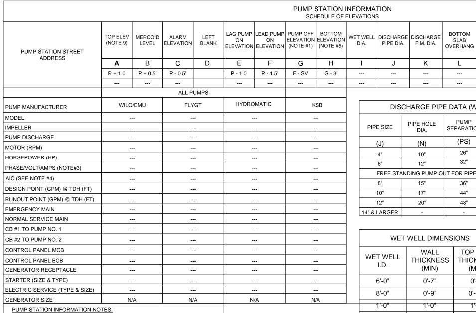
DISCHARGE PIPE DATA (WITHIN WET WELL) HATCH SIZE PUMPOUT SEPARATION (MIN.) SIZE (PO) (PS) 26" 36"x48" 4" 32" 6" 36"x60" FREE STANDING PUMP OUT FOR PIPE SIZES GREATER THAN 6" 17" 44" 10" 12" 14" & LARGER 14" & LARGER
