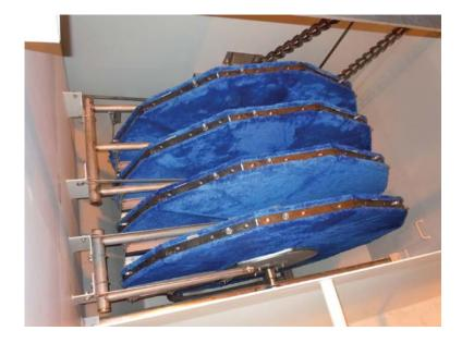
**DESCRIPTION:** Fixed filter disk used in removing solids from liquids. Structure allows for high efficient filtration, low backwash volume and is a reusable element.
