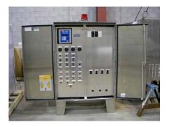
DESCRIPTION: Pump Station Electrical and Control Panel including (RTU) and Variable Frequency Drives (VFD). See Section 433 of the current JEA Standards for specifications and requirements.
