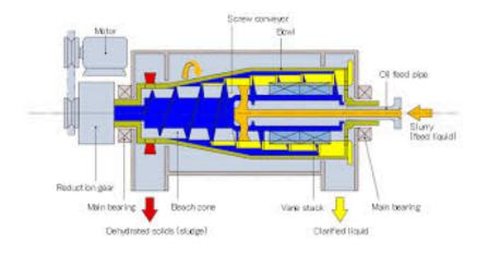
**DESCRIPTION:** Used for sludge dewatering needs. The centrifuge can remove the water content from sludge by rotating it at a high speed, so sludge can be disposed of in a cost-efficient manner.
