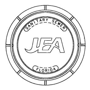
DESCRIPTION: Manhole Frame and Cover (with rubber "T" Gaskets). See Section 427 of the current JEA Standards for specifications and requirements.
