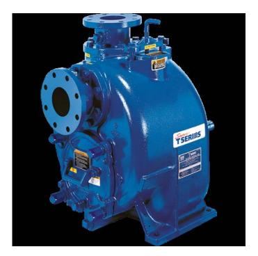
**DESCRIPTION:** Designed with a large reservoir surrounding the pump casing which allows the pump to retain enough water internally to not need additional manual priming.
