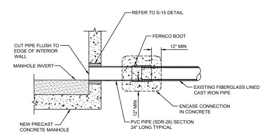
EXISTING CAST IRON PIPE WITH LINER
