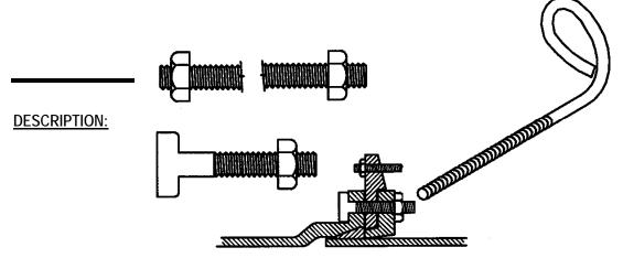
Mechanical Joint Fasteners. See Chapter III. 1. - Section 350 of the current JEA Standards for specifications and requirements. See Chapter VI. 1. - Section 701 for Reclaimed Water specifications and requirements.
