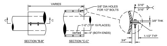
MATERIAL: PIPE - ATSM A53, GRADE B, ERW, STD WALL, CARBON STEEL PLATE - STM A36, GRADE B, CARBON STEEL (THICKNESS AS NOTED)
