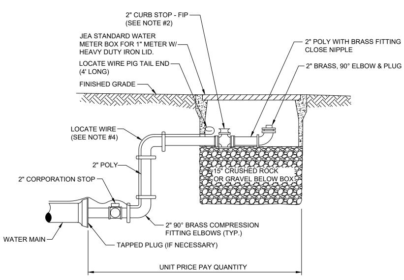
1. PIPE SHALL BE POLYETHYLENE. FITTINGS SHALL BE BRASS.
