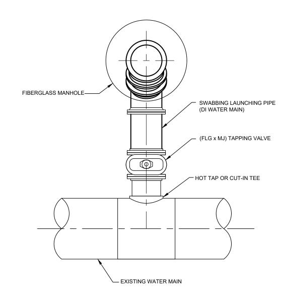
1. FOR HOT TAP CONNECTIONS ON EXISTING WATER MAINS 10" DIAMETER AND GREATER, Diameter of tapping valve and pig launching pipe shall be one nominal size LESS than existing water main.
