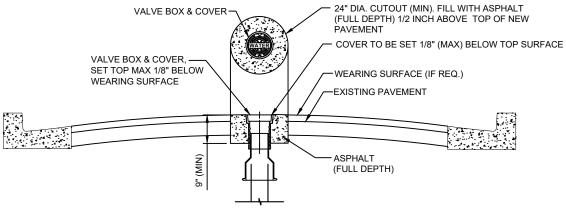
PROVIDE FULL DEPTH ASPHALT 1/2 INCH ABOVE TOP OF NEW PAVEMENT LEVEL, TO ALLOW FOR FUTURE ASPHALT MATERIAL COMPACTION. PLACE AND COMPACT ASPHALT IN 2" (MAX) LIFTS.
