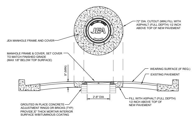
PROVIDE FULL DEPTH ASPHALT 1/2 INCH ABOVE TOP OF NEW PAVEMENT LEVEL, TO ALLOW FOR FUTURE ASPHALT MATERIAL COMPACTION. PLACE AND COMPACT ASPHALT IN 2" (MAX) LIFTS.
