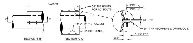
MATERIAL: PIPE - ATSM A53, GRADE B, ERW, STD WALL, CARBON STEEL PLATE - STM A36, GRADE B, CARBON STEEL (THICKNESS AS NOTED)
