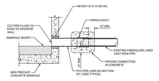
EXISTING CAST IRON PIPE WITH LINER
