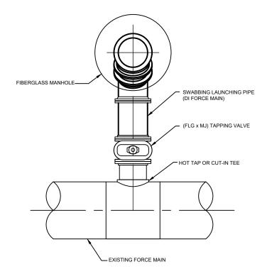
1. FOR HOT TAP CONNECTIONS ON EXISTING FORCE MAINS 10' DIAMETER AND GREATER, DIAMETER OF TAPPING VALVE AND PIG LAUNCHING PIPE SHALL BE ONE NOMINAL SIZE LESS THAN EXISTING FORCE MAIN.
