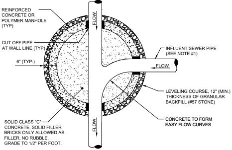
THE ANGLE BETWEEN ALL INFLUENT FLOW CHANNELS AND EFFLUENT PIPE SHALL BE BETWEEN 90° - 180° UNLESS OTHERWISE APPROVED BY JEA.
