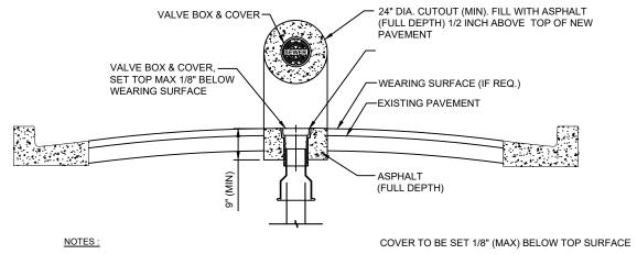
PROVIDE FULL DEPTH ASPHALT 1/2 INCH ABOVE TOP OF NEW PAVEMENT LEVEL, TO ALLOW FOR FUTURE ASPHALT MATERIAL COMPACTION. PLACE AND COMPACT ASPHALT IN 2" (MAX) LIFTS.
