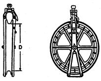
Figure 3. Sheave Diameter
