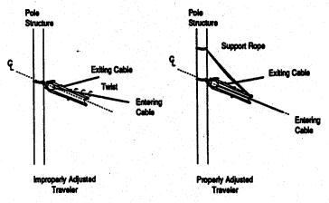
Figure 1. Proper Traveler Adjustment.
