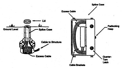
Figure 7. Underground and Pole Mounted Housing
