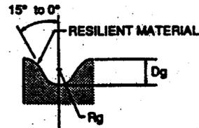
Figure 4. Sheave Groove
