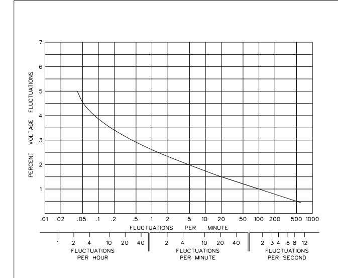
THE CUSTOMER SHALL NOT BE ALLOWED TO IMPOSE VOLTAGE FLUCTUATIONS ABOVE FIVE (5) PERCENT ON THE JEA SYSTEM EXCEPT UNDER EXTREME CIRCUMSTANCES. FOR APPROVAL, CONTACT THE JEA DISTRIBUTION PLANNING AND ANALYSIS SECTION.
