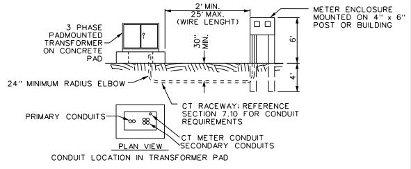
NOTE: METERING CURRENT TRANSFORMERS LOCATED INSIDE PADMOUNTED TRANSFORMER, APPLICABLE ONLY WHEN A SINGLE PADMOUNTED TRANSFORMER PROVIDES SERVICE TO A SINGLE CUSTOMER. REFERENCE SECTION 4.05. \*
