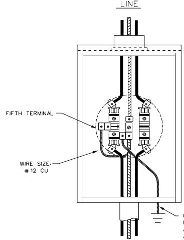
GROUND METER SOCKET IN ACCORDANCE WITH NEC AND LOCAL INSPECTION AUTHORITY REQUIREMENTS
