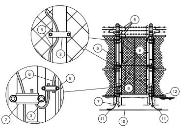
FENCE GROUNDING DETAIL - CORNER POST NOT TO SCALE
