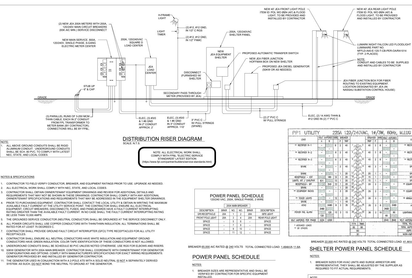
SHELTER POWER PANEL IS DIAGRAMMATIC ONLY. CONTRACTOR SHALL VERIFY PANEL CONFIGURATION WITH SHELTER MANUFACTURER
