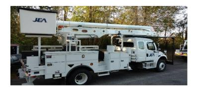
1.5. Category C 45' to 50' Derrick Digger (18" AUGER): Example Altec DM47, Altec DH50 or Equal
