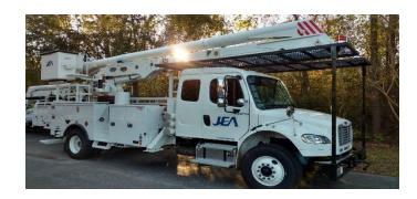
1.4. Category C 55' to 60' TWO MAN / MATERIAL HANDLER Bucket Trucks: Example Altec AA-55E with 2000 LB Capacity JIB or Equal
