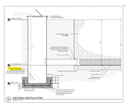
**Answer:** The Pump and outflow pipe are "Future". They do not need to install any pump or controller. The Scope of Work shall include the Wet Well as an inspection point but won't include any pump thus "Future". It will allow for a more standardize design where it could allow for a pump in the future if the CI Agent material gets clogged. The installation of this well allows for a visual indication that the containment is still operational.
