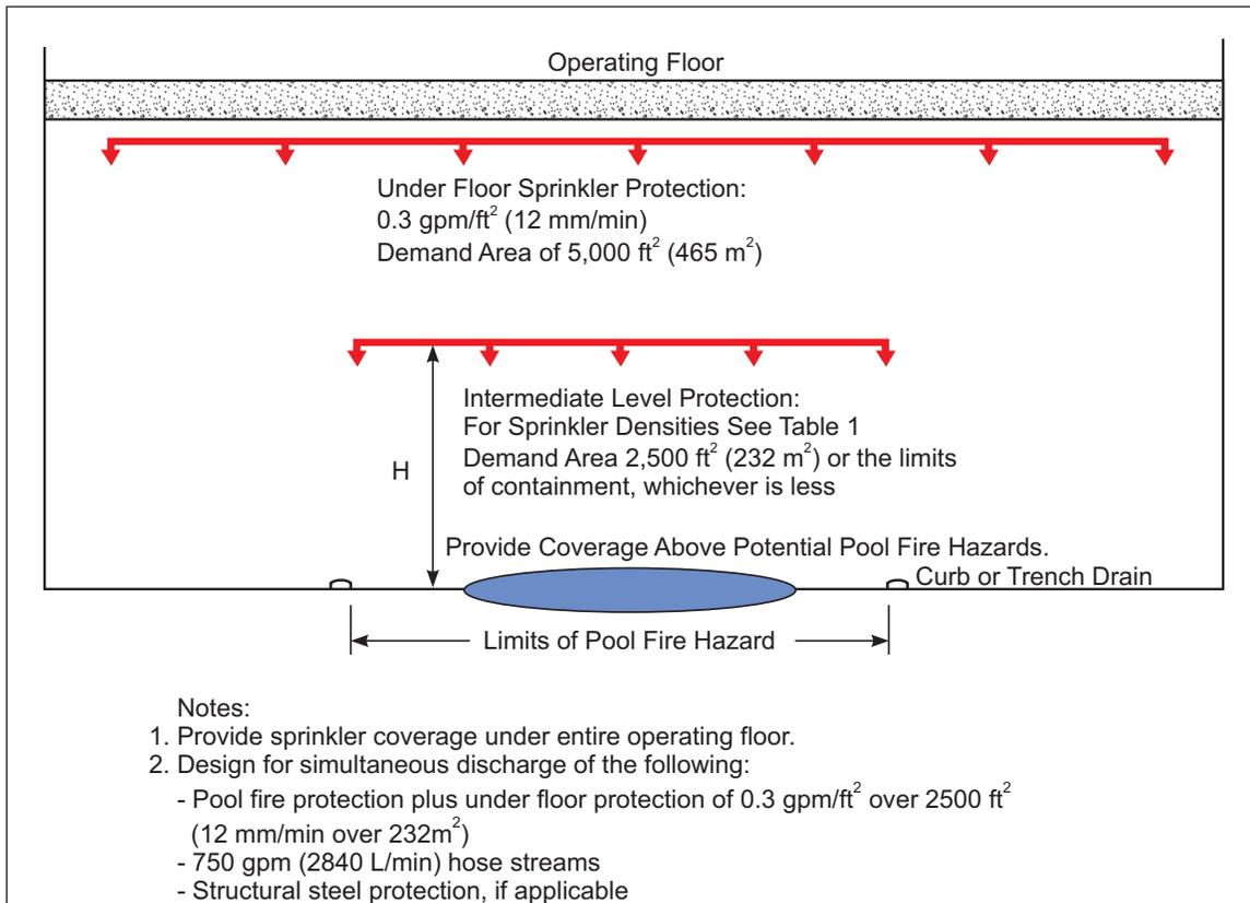
Fig. 9b. Optional protection for turbine buildings with solid operating floors higher than 30 ft (9.1 m)
