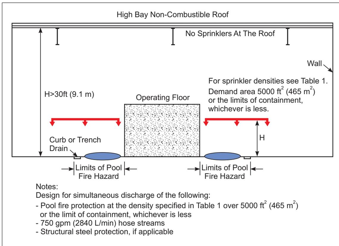
Fig. 9g. Local protection for solid pedestal designs
