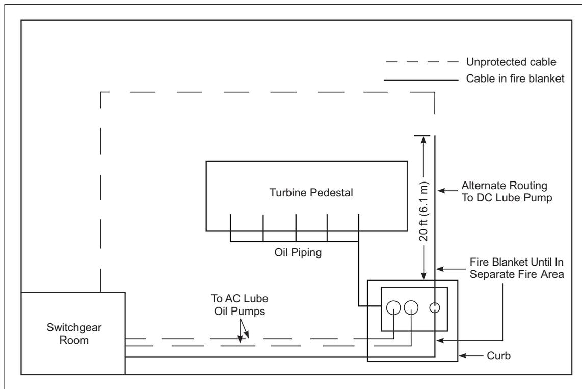
Fig. 3. Cable protection for dc lube oil pump
