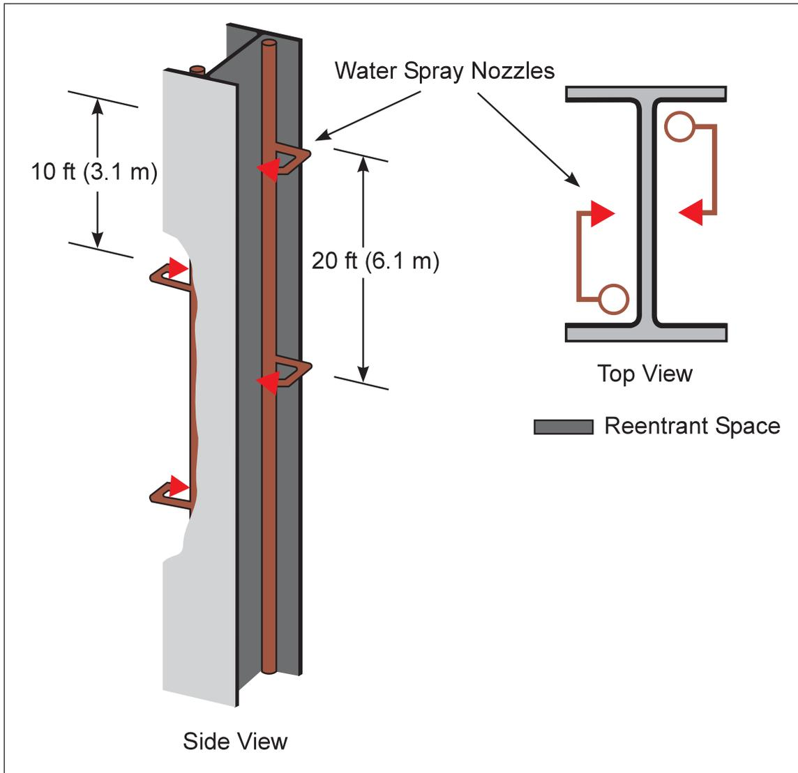
Fig. 1b. Water spray protection for steel columns
