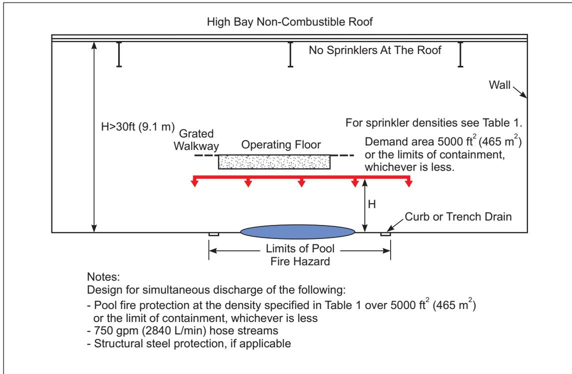
Fig. 9e. Local protection for island type turbine buildings
