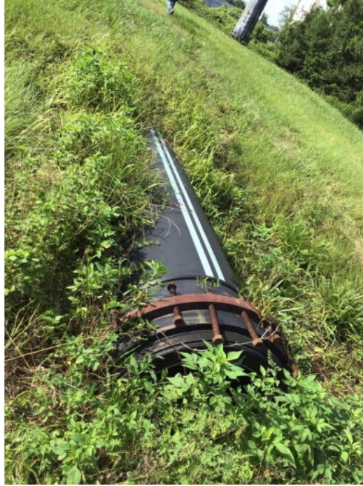
Photo 2: Failed Reclaimed Water Main HDD (exposed pipe in T-Line north of JTB)
