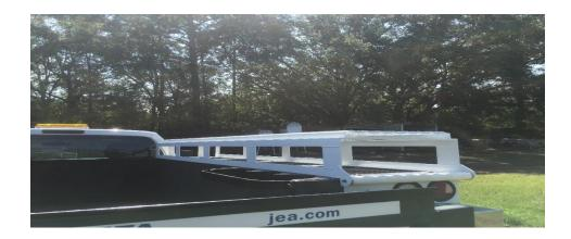
1600 LB Capacity Lift Gate: MAXON ME2 SERIES 49" X 27", ALUMINUM with Dual Hydraulic Cylinders and Remote Control Pendant.
