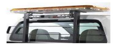
11.12 **LED GO LIGHT (Remote Controlled):** Model # 20074, Radioray LED. Hard Wired / Mounted to the **JV WeCan Series Super LED** MODEL **JV2A Light Bar.** No Exposed Wires
