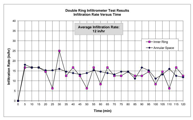
**Comments:** Rings were re-filled when needed due to the infiltration rates measured in the field.
