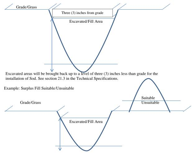
This shows having surplus fill for "Suitable" and "Unsuitable" usage. In this case "Suitable" will be used to back fill the excavated area, the "Unsuitable" will be disposed of as per section 42 item number 18.
