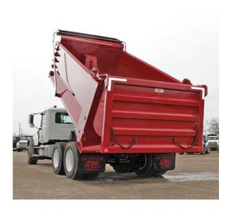
14.2 **TARP SYSTEM:** Aluminum Automatic TELESCOPING Tarp System.
