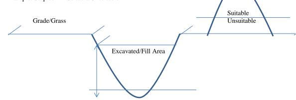
This shows having surplus fill for "Suitable" and "Unsuitable" usage. In this case "Suitable" will be used to back fill the excavated area, the "Unsuitable" will be disposed of as per section 42 item number 18.
