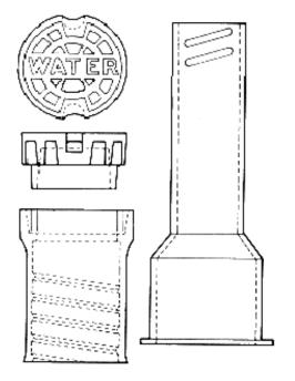
**DESCRIPTION:** Valve Box and Cover. See Section 351 of the current JEA Standards for specifications and requirements. See Section 702 for Reclaimed Water specifications and requirements.
