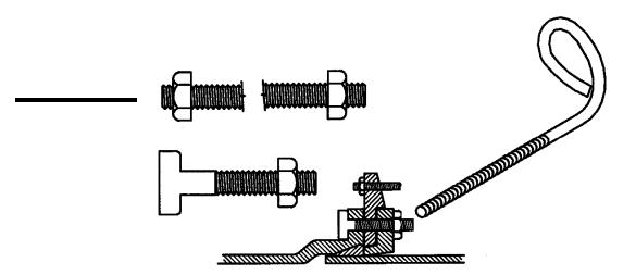
**DESCRIPTION:** Mechanical Joint Fasteners. See Chapter III. 1. - Section 350 of the current JEA Standards for specifications and requirements. See Chapter V. 1. - Section 701 for Reclaimed Water specifications and requirements.
