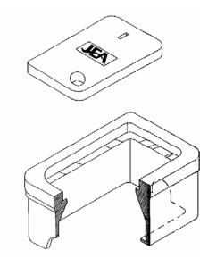
DESCRIPTION: Meter Box. See Chapter III. 2. - Section 351 of the current JEA Standards for specifications and requirements. See Chapter V. 2. - Section 702 for Reclaimed Water specifications and requirements.
