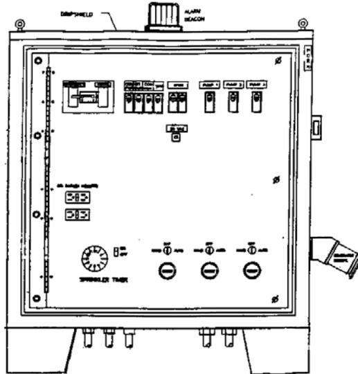
**DESCRIPTION:** Pump Station Electrical and Control Panel including (RTU). See Section 433 of the current JEA Standards for specifications and requirements.
