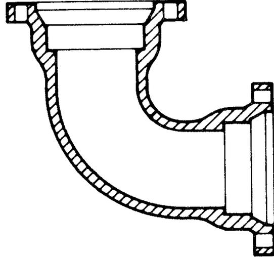
**Note:** Mechanical joint, 90-degree bend & fittings, shown as example only (for additional joints, see specifications).
