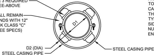
PROVIDE COLD ROLLED STEEL TIE RODS FROM THE END OF THE STEEL CASING PIPE TO THE FIRST JOINT OF PIPE OUTSIDE THE CASING. THE RODS ARE TO BE WELDED TO THE CASING AND CONNECTED TO A BELL TYPE CLAMP ON THE PIPE. (TYPICAL EACH SIDE). SEE TABLE BELOW FOR THE MINIMUM NUMBER OF TIE RODS REQUIRED AT EACH END, TIE ROD SIZE AND QUANTITY.
