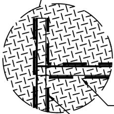
CONSTRUCT WITH 1 1/4" ANGLE (STEEL 3/16" THK), 12" LONG WITH CENTER STIFFENER
