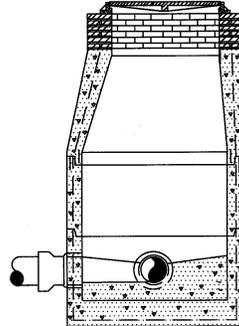
**DESCRIPTION:** Manhole and Accessories. See Section 427 of the current JEA Standards for specifications and requirements.
