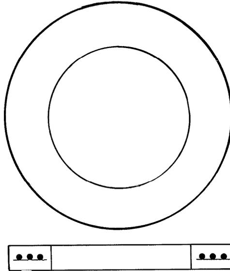
**DESCRIPTION:** Manhole (adjustment rings) Collars. See Section 427 of the current JEA Standards for specifications and requirements.
