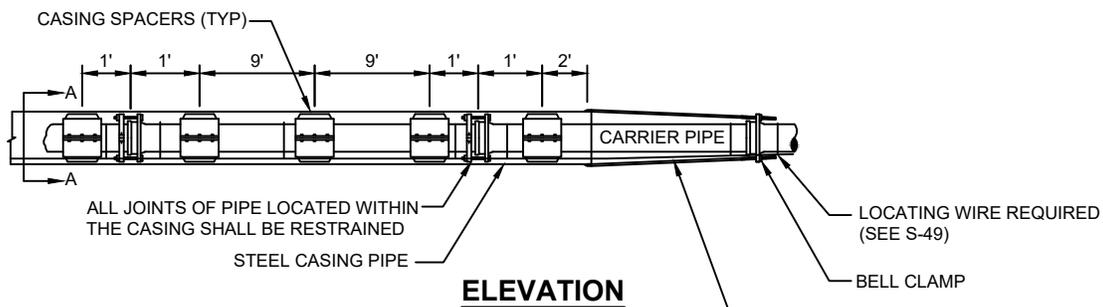
CASING SPACER 2 OR 3 REQUIRED PER JOINT OF PIPE SEE-ABOVE
