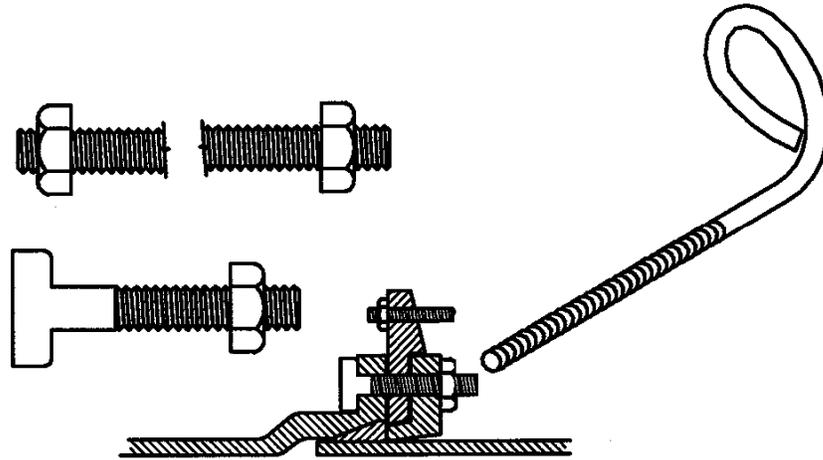
**DESCRIPTION:** Mechanical Joint Fasteners. See Chapter IV. 3. - Section 429 of the current JEA Standards for specifications and requirements.
