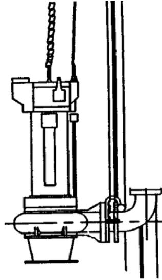
**DESCRIPTION:** Wastewater Pump. See Section 433 of the current JEA Standards for specifications and requirements. It is intended that JEA approved material list shall be considered acceptable, unless new technology exist or if it is in the best interest of JEA to revise the approved material list.
