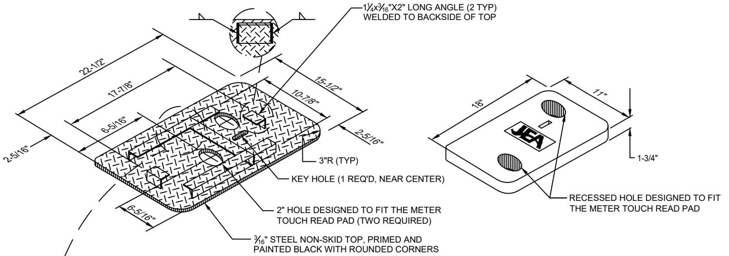
PROVIDE 2" PVC PLUGS TO CLOSE HOLES WHICH ARE NOT USED OR WHERE NO METER IS INSTALLED DURING THE CONSTRUCTION PERIOD (NOT-IN-USE SERVICE).
