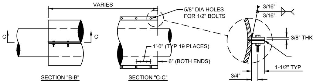
MATERIAL: PIPE - ATSM A53, GRADE B, ERW, STD WALL, CARBON STEEL
